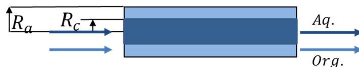
Figure 1 Schematic of core-annular flow
